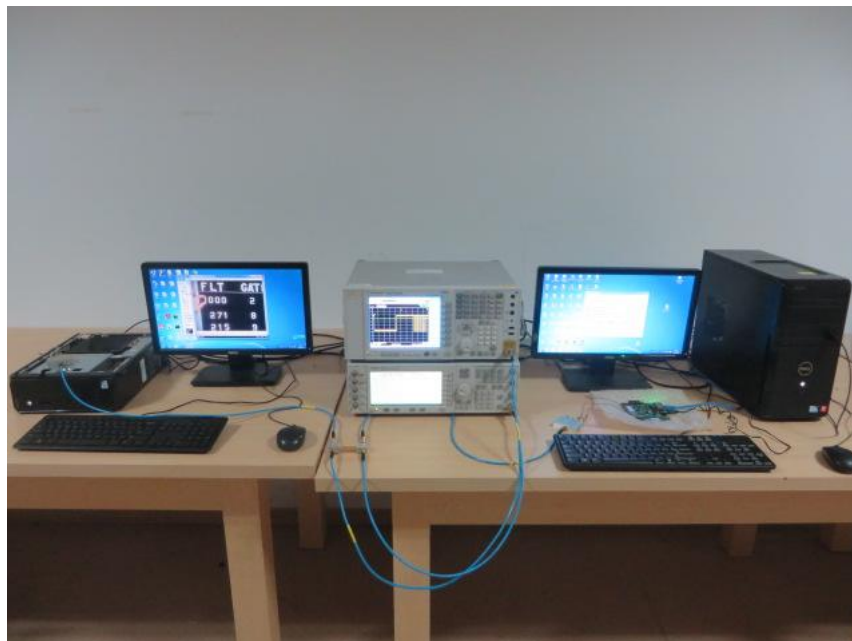
DFS Test Set-up Photo for Master Device - Set-up A
